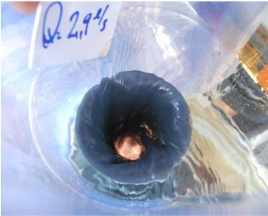
**Figure 1:** Presence of a vortex at a discharge of 2.9 l/s
