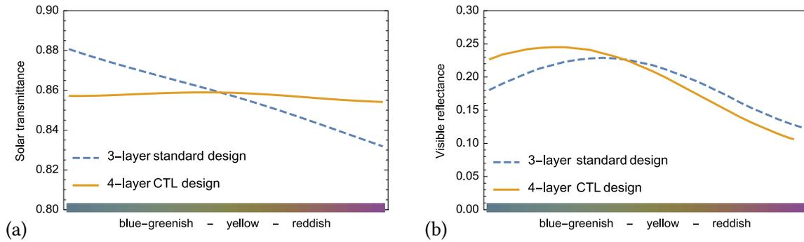
Figure 3: Simulated solar transmittance and visible reflectance of the standard and the CTL design. The reflection colour of both design types follow the same trajectory in the  $a^*b^*$ -plane, which is indicated on the x-axis in form of calculated colours in the CIELAB system.
