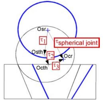
If we explicit the case of the spherical joint, we obtain the following torsor  $[\tau_{\text{spherical joint}}]_{\text{Osth}}$  (between Osr and Ocr), calculated at point Osth (Osth is the theoretical centre of the sphere, Osr is the real centre of the sphere, idem for the points Octh and Ocr characterising the cone):
