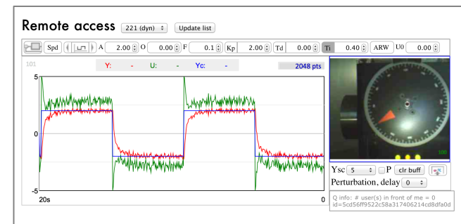
Figure 1: The user interface composed of a command strip through which the students can control the lab, an oscilloscope screen, and a video feed as shown in the MOOC
