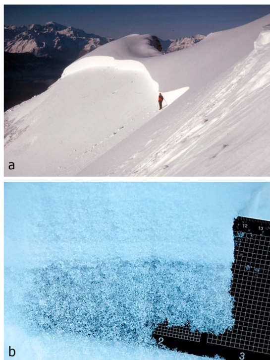
Figure 1. (a) Crown fracture of a dry-snow slab avalanche in La Sionne, Switzerland ©SLF. (b) Depth hoar weak layer.
