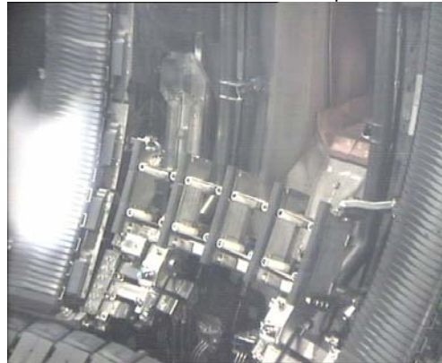
AE antennas as installed in-vessel in June 2005.
