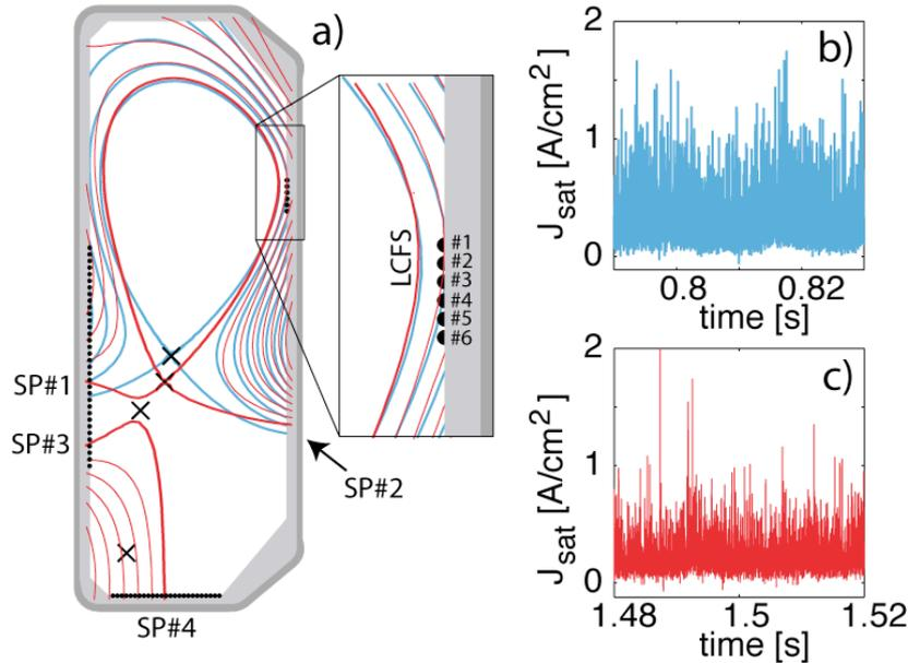
FIG. 4: a) Plasma shapes for the SN (blue) and SF+ (red) configurations with LPs #1-#3 in the SOL. The numbering of the different strike points (SP) is indicated. Examples of measured  $J_{\text{sat}}$  in the SN phase b) and later in the SF+ phase c).
