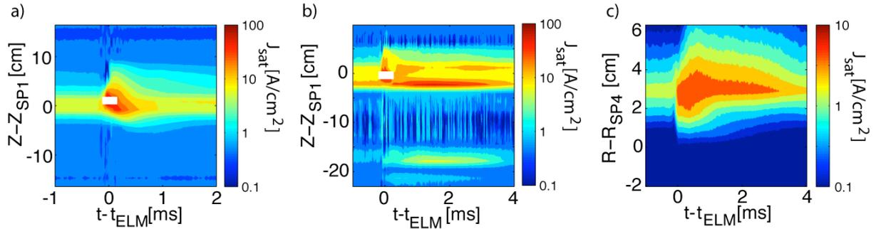
FIG. 7: 2D profiles of  $J_{sat}$  versus  $t-t_{ELM}$  for the target zone of SP1 a) in the SN configuration b) in the SF+ configuration and for the target zone of SP4 in SF+ configuration.
