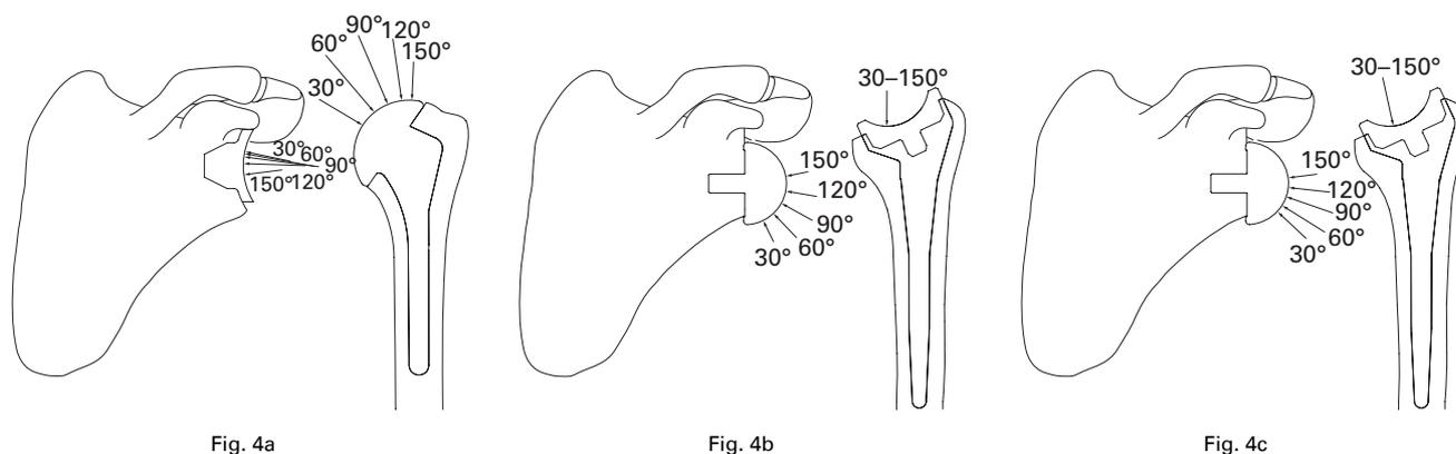
Diagrams showing the direction of the glenohumeral joint force, on the glenoid and humeral side, every 30° of abduction in the scapular plane, for a) the anatomical prosthesis, b) the reversed prosthesis without any rotator cuff muscle, and c) the reversed prosthesis without supraspinatus only.
