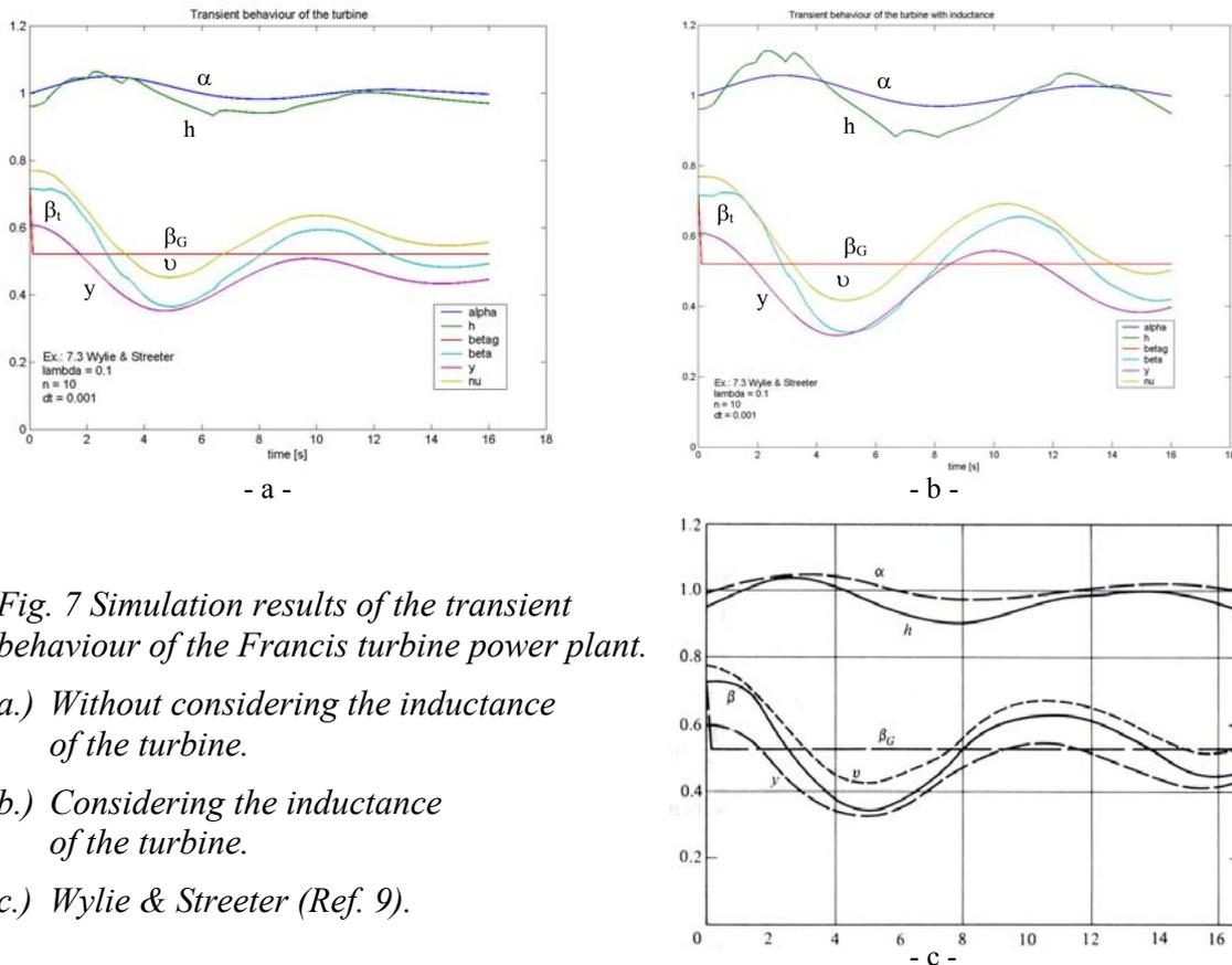
Fig. 7 Simulation results of the transient behaviour of the Francis turbine power plant.
