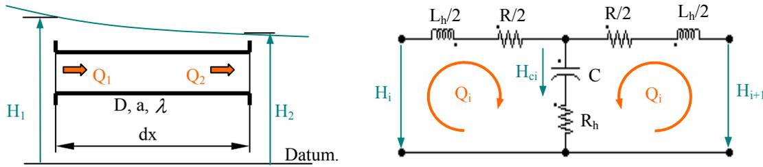
Fig. 1 Crossflow section of a pipe modelled using impedance method.
