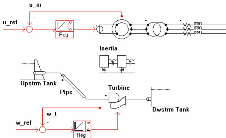
Fig. 5 Modelling with SIMSEN of a power plant including a Francis turbine coupled to a generator.
