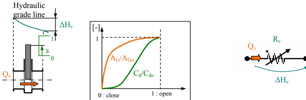
Fig. 2 Valve modelled using impedance method.
