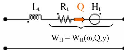
Fig. 4 Simplified impedance model of the Francis turbine.
