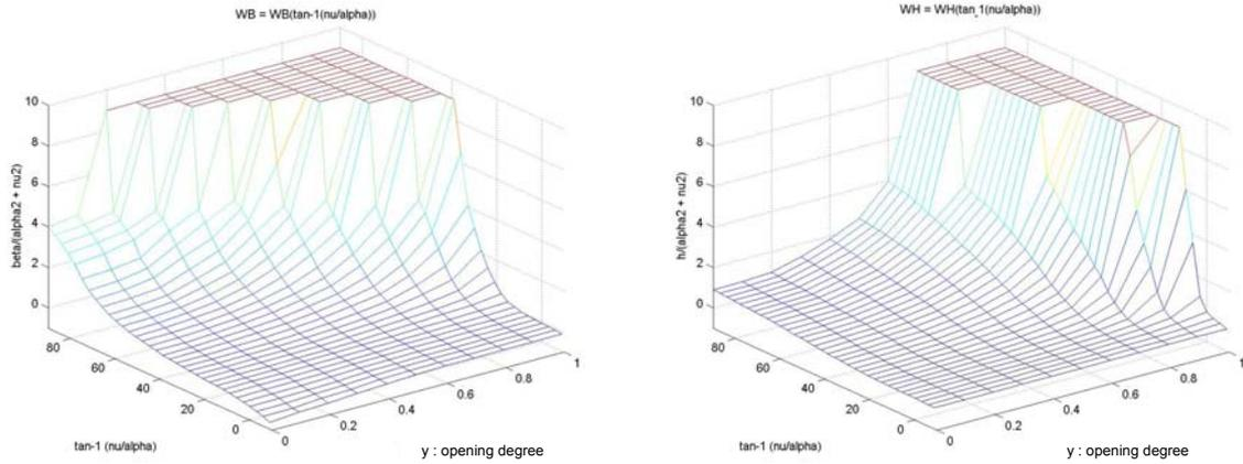
Fig. 6 Characteristics  $W_B$  and  $W_H$  of the turbine.
