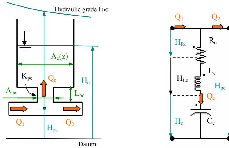
Fig. 3 Surge tank modelled using impedance method.
