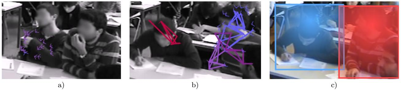
**Figure 3: Motion detection and grouping.** *a)* Individual motion vectors shown as purple arrows *b)* Motion vectors grouped over time into motion tracks which can be assigned to an individual *c)* Marked student areas and centres of Gaussian probabilities which model the probability of motion belonging to each student.
